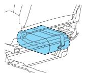
To replace the temporary mobility kit, open the Velcro<sup>®</sup> strap on the bag and slide the bag back under the driver's seat. Wrap the strap over the rear frame bar, loop it through the buckle and secure the bag to the seat frame.
